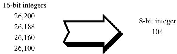
This conversion is what makes the BYTE download format less accurate than the WORD format.
